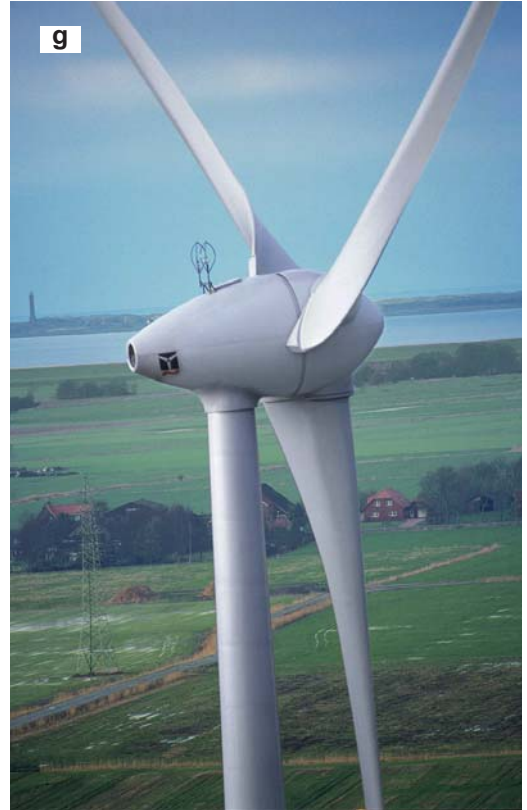
Figure 7(f–h). Examples of products that embody balsa: the hull and deck of the Douglas Marine Spiderman (f); end-grain balsa cores are used in rotor blades for wind turbines (g) where high shear and compression strengths are required; historically, the de Havilland Mosquito bomber of World War II incorporated balsa into its famous wooden construction (h). (Photos: a–f, Alcan Baltek; g, ENERCON; h, The Australian War Memorial)
