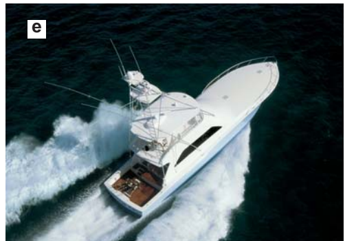
Figure 7(a–e). Examples of products that embody balsa: many vehicles include panels with balsa cores, such as the floor panels of the Cadillac XLR (a), structural bodywork of the Toyota IMTS bus (b), the cab floor of the Kenworth T2000 truck (c), the hull and deck of the Dehler 47 yacht (d) and various sections of the Viking 74 sports fishing boat (e).
