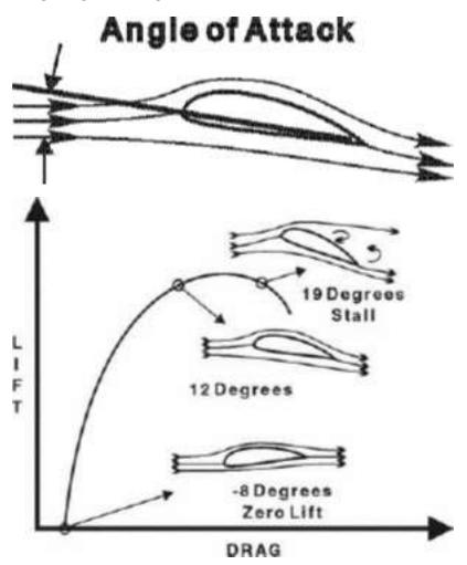
It is the angle the wind makes with the wing (relative wind). As the angle of attack increases, so more lift is generated -but only up to a point until the smooth airflow over the wing is broken up and so the generation of lift cannot be sustained. When this happens, the sudden loss of lift will result in the airplane entering into a stall, where the weight of the airplane cannot be supported any longer
