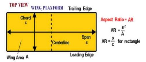
ASPECT RATIO the Ratio of the wing span to the wing's chord length(c).
