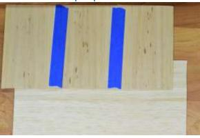
On this particular project we have to laminate our balsa together. We will take a 1/16" balsa and laminated one sheet one way and next sheet 90° from grain direction of the first sheet. This way we have created a balsa plywood. The only other thing you need to do is cut your other 1/16" balsa for the wings and the aileron on the tail.
