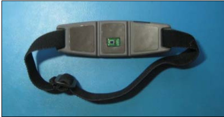
BALSM 2 nd Year Pulse Ox Sensor Prototype - Sensor Side
