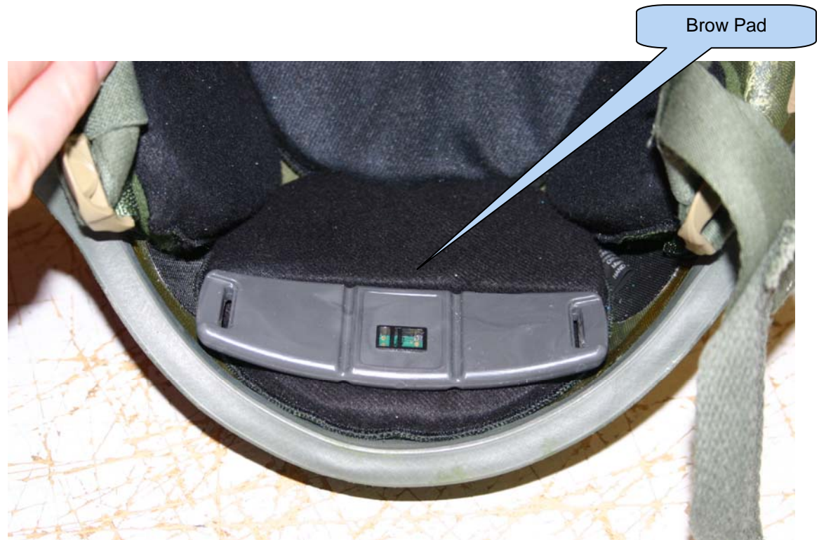
Photo of custom brow pad with BALSAM 2 nd year pulse oximetry sensor model.
