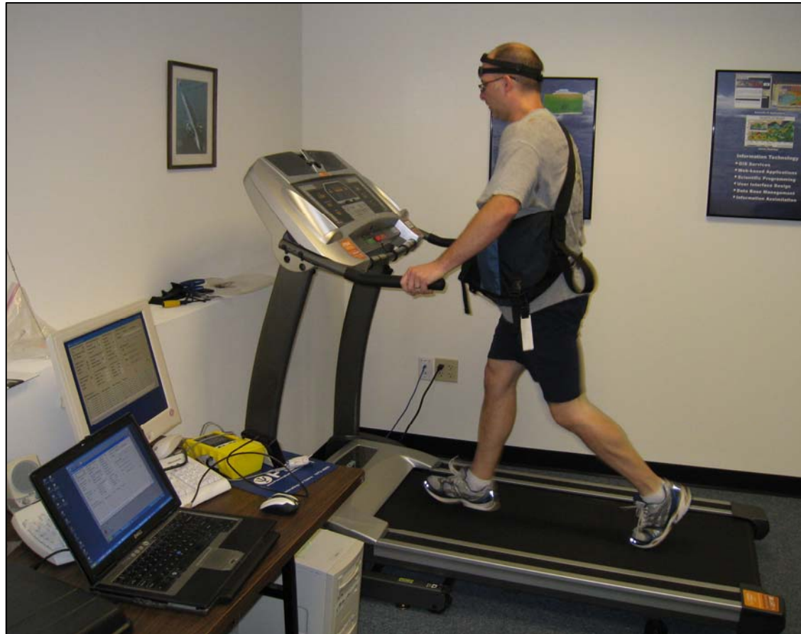
Testing with both 1 st and 2 nd year BALSAM pulse ox sensors.
