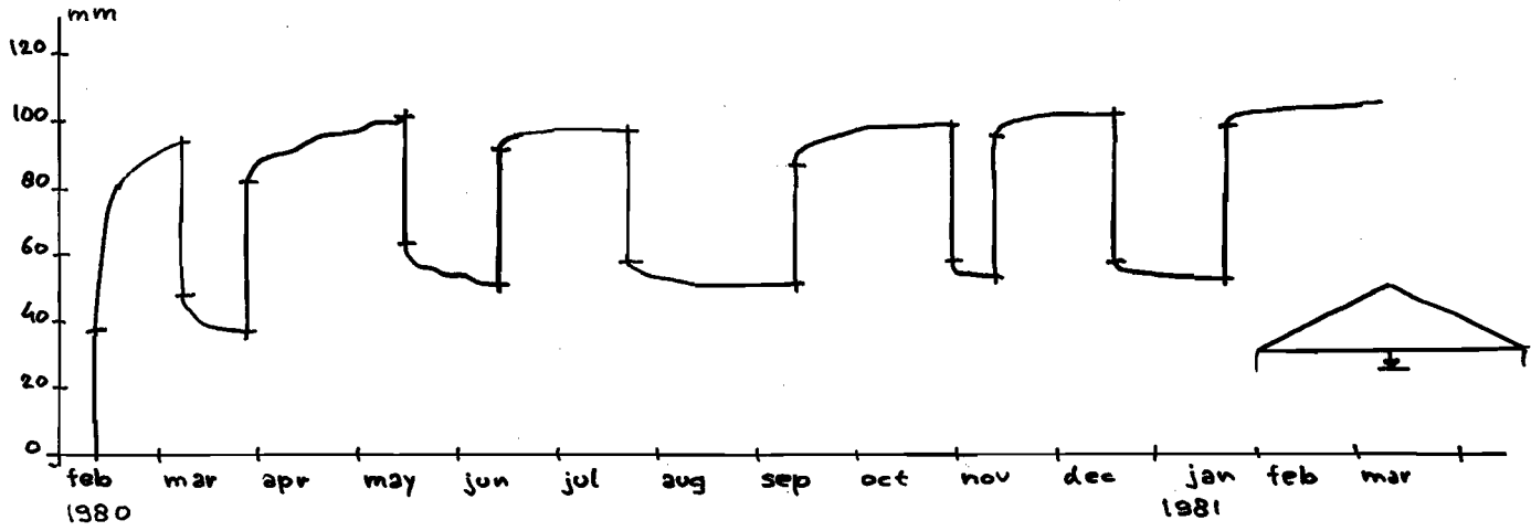
Fig. 5.8.19. Creep and recovery, truss no. 5
