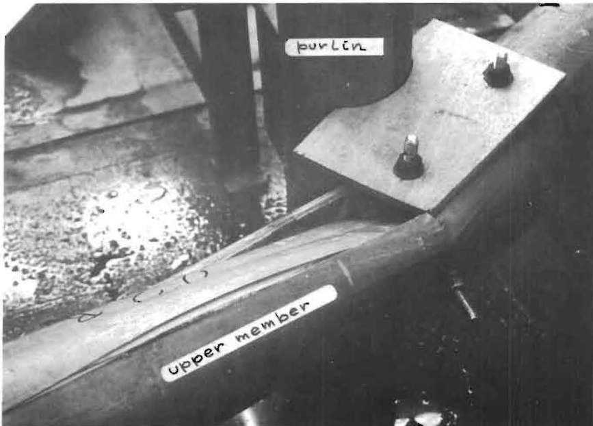
Picture 5.6.2. Joint type 7.6., specimen B-2, failure at purlin 1.
