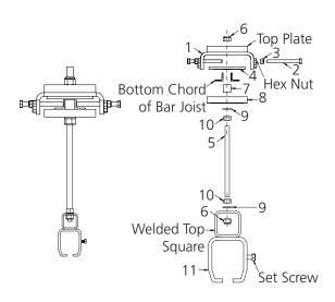
NOTE: The spacer plate (4) is only required for bar joist hanger assembly 8-0676. 700 Series Plain Track uses 3/4-inch diameter hardware. Torque 3/4-inch diameter hardware to 151 foot-pounds.
