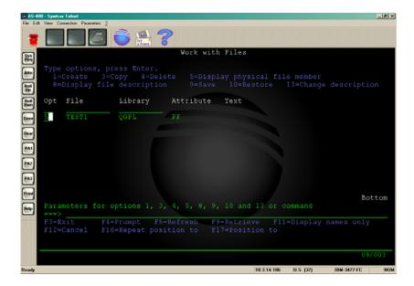
TAB to the start of the line containing TEST1 and enter 5, press ENTER.
