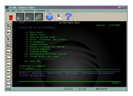
❖ The first step is to start the trace, this can be done by typing **STRSST**
