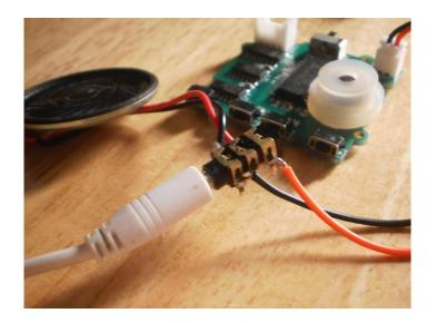
The audio jack shown here is the stereo jack extension cable attached, but the output will only be mono from the sound recorder. What we can do is to connect just only 1 (the farthest terminal) to the + pin of the sound recorder and then the – pin will be connected to the nearest terminal of the plug.
