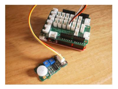
Connect the Twig PIR Motion Sensor to port 10 of the Stem Base Shield.
