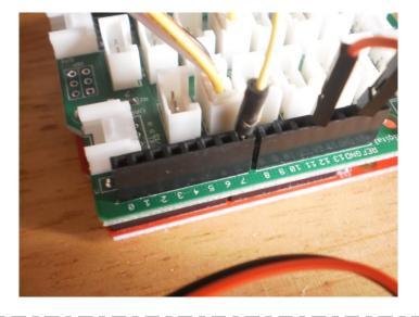
Connect the INT pin from the touch sensor to the PIN 7 of the Stem Base Shield.
