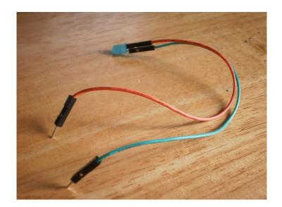
The hookup wires shown here are 1 pin female jumper wires. But if you don't have one, breadboard jumper wires are good but you will have to solder on to the leads of the LED. Colorcoded also here are RED for the input voltage (or signal) and GREEN for ground.
