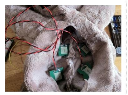
Place them flat inside of the dog with the feelers faced against its fur. From the illustration here, we can see that the backside of the feelers is the one that would be visible. You can go ahead and experiment on the positioning of the feelers.
