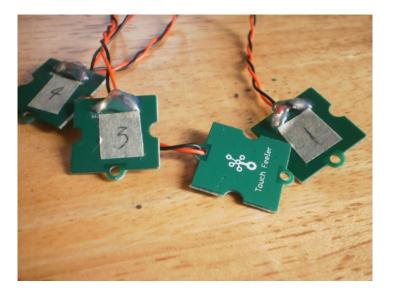
Matching the ports on the sensor, place a label on each of the touch feelers:
