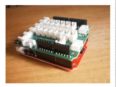
Stack up the Stem Basic Shield on top of the Seeeduino. Make sure that it is fit snugly and rests flat with the Seeeduino.
