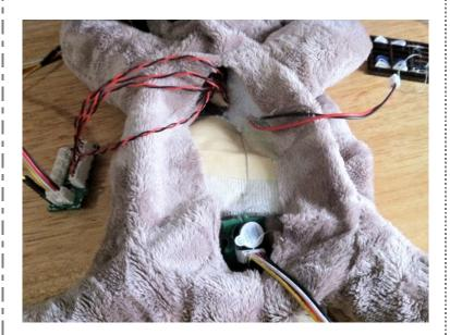
We can place the buzzer anywhere we want, and on the illustration here, the buzzer is sewn near the back of the dog.
