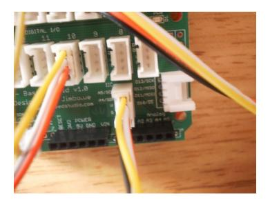
Then connect the grove cable to any of the 2 I2C ports in the Stem Base Shield.
