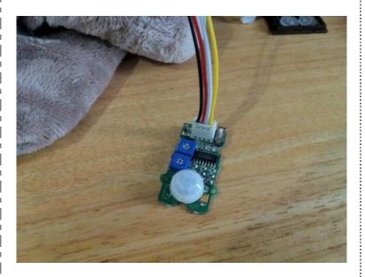
Then let us now sew the Twig Motion Sensor on the dog's neck. This sensor has 3 holes on it and we can use them as the anchoring points.
