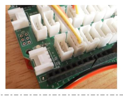
Connect the Sound Recorder to port 2 of the Stem Base Shield.
