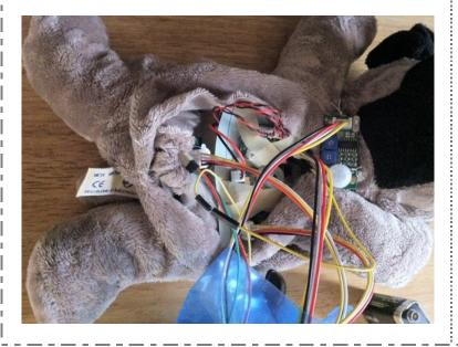
Put in our I2C Touch Sensor board/Sound Recorder board inside the dog, with the cardboard resting on top of the beanie bag/bubble wrap.
