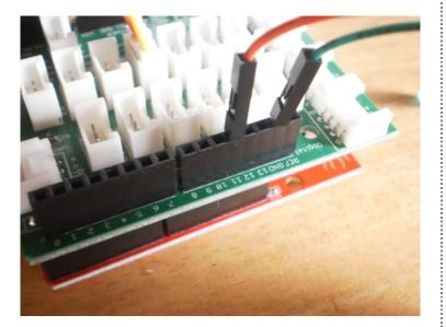
Then connect the ground wire (GREEN) to the GND pin and the input voltage (RED) to pin 11 along the **digital** pins of the Stem Base Shield.
