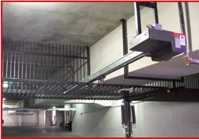
The solid steel frame and belt-driven gear box make this Operator one of the quietest in the market today (shown with optional cover).
