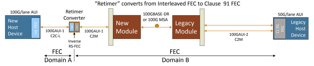
Note: Above is akin to PAM4-based host talking to CAUI-4 QSFP28 module through KP/KR FEC converter chip
