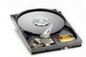
A hard disk is a set of stacked disks. Each disk has data recorded electromagnetically in concentric circles, or tracks, on the disk Hard Drive Types
