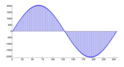
Figure 1.2: Sine wave with 256 samples
