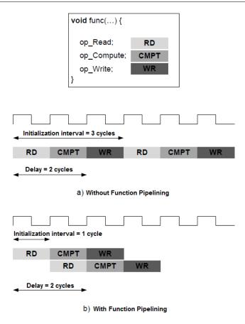
Figure 2.44: Function Pipelining Behavior
