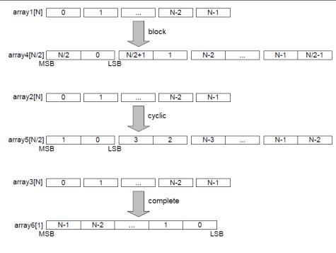
Figure 2.53: Array Reshaping
