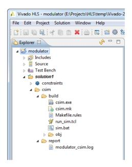
Figure 2.19: Explorer window with C Simulation Output Files
