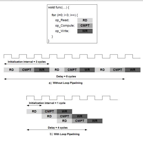
Figure 2.45: Loop Pipelining Behavior
