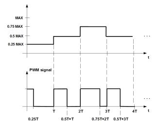
Figure 1.1: Example of the PWM signal
