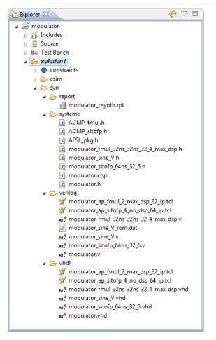
Figure 2.28: Explorer window with C Synthesis Output Files
