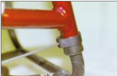
Fig. 1-D Allen wrench used to adjust footplate on Action™ Pro-T.
