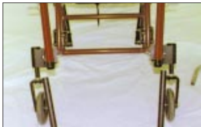
Fig. 1-E The footplate tubes do not line up with the openings in the front of the frame in wheelchairs with tapered front rigging.
