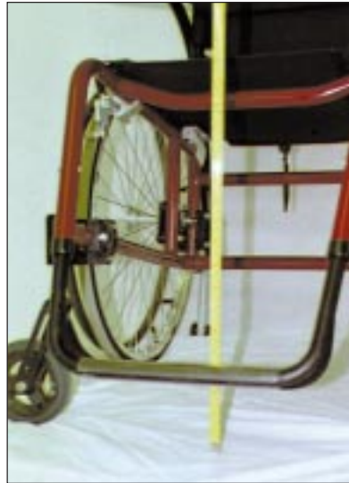
Fig. 1-A Two inches of footplate-to-floor clearance needed.
