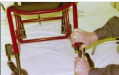
Fig. 1-F It will take some force to align the footplate tubes with the openings in the front frame.
