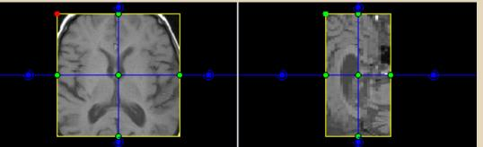
isotropic imaging - all 3 sides (x, y, z) of the voxel have equal size
