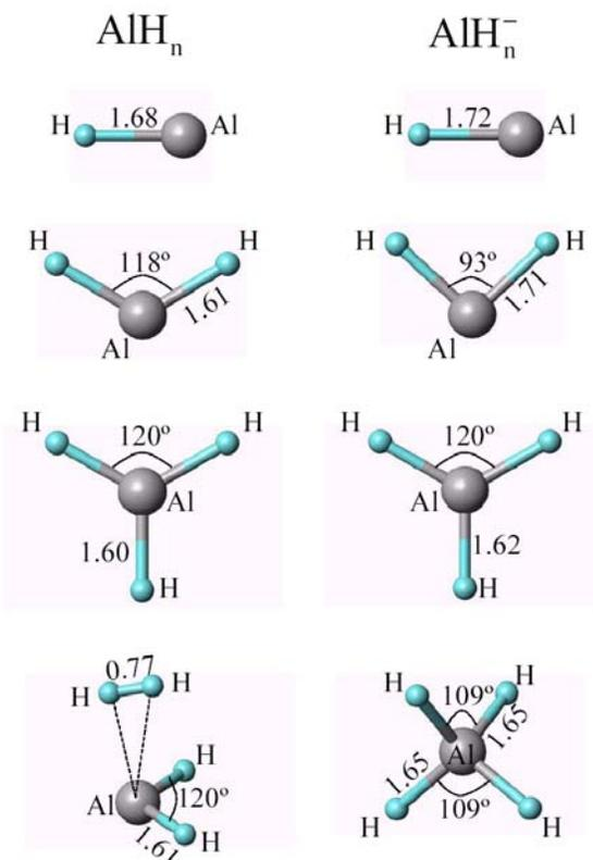
First principles density functional theory shows that neutral AlH<sub>4</sub> dissociates into AlH<sub>2</sub> + H<sub>2</sub> but that ionized AlH<sub>4</sub><sup>-</sup> tightly binds 4 hydrogens.
