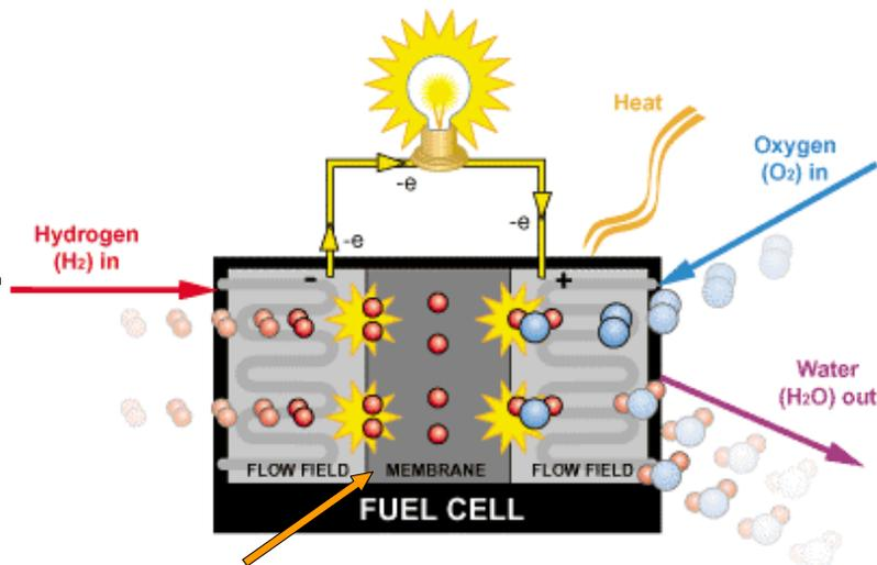
Membrane conducts protons from anode to cathode
