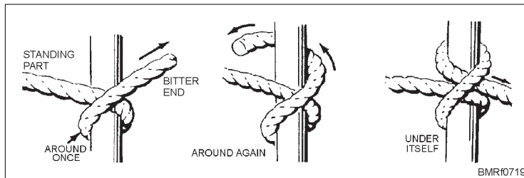
Figure 7-19.—Tying a clove hitch.
