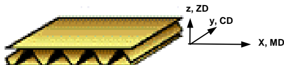
Figure 1. Single-wall corrugated board.
