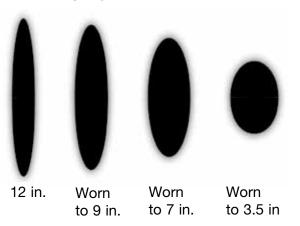
Example: When a tip that had a 12-inch fan pattern is reduced to a 9-inch fan when worn, it will output 40% more paint on 25% less area. Overlapping to achieve a consistent mil thickness becomes impossible. The chart above illustrates the effects of a worn tip on a spray pattern.
