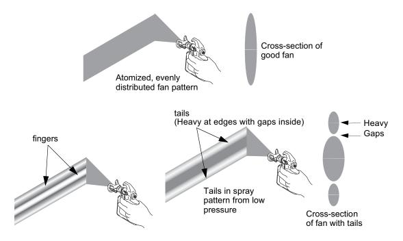
**Note**: If the maximum pressure of the sprayer is not enough to achieve a good spray pattern, a spray tip with a smaller orifice should be used. To test the quality of the spray pattern, test patterns should be sprayed on scraps of cardboard or other waste material.
