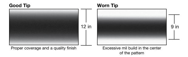
If abrasive materials are sprayed at too high of pressure, the spray tip will wear a lot faster, wasting both paint and money.
