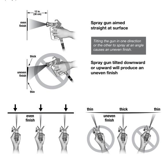
The spray gun should move across the surface with the wrist flexed to keep the gun pointed straight at the surface. "Fanning" the gun to direct the spray at an angle will cause an uneven finish.
