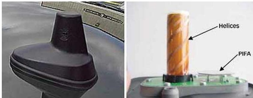
5. This antenna design is a combination of quadrifilar and PIFA structures.
