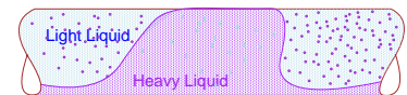
Fig. -5.4: Plug flow in horizontal tubes when the liquids flow is faster slow.
