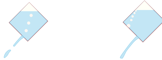
Fig. -5.10: Counter-current flow in a can (the left figure) has only one hole thus pulse flow and a flow with two holes (right picture).
