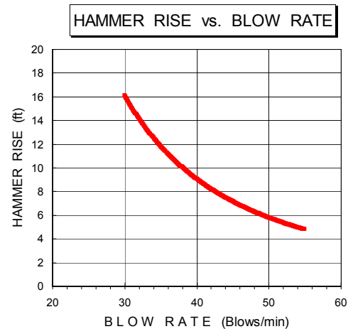
Fig. 9.7 Hammer rise (ft) as a function of blow-rate (BPM) (single-acting diesel hammer)
