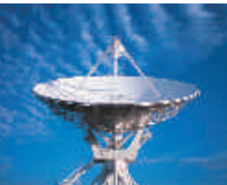
Radio telescopes pick up electromagnetic waves with a wavelength between 3 cm and 6 m
