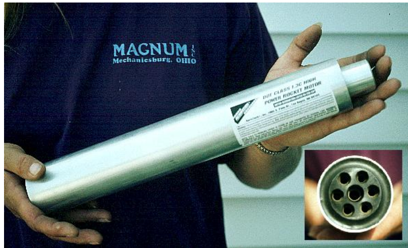
Typical single use high power rocket motor
