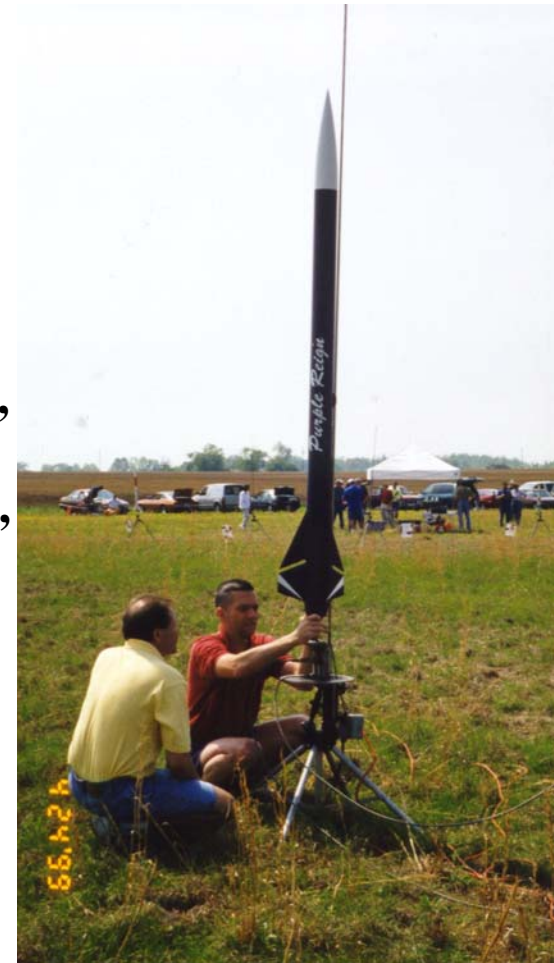
Myself and Oscar Valent preparing my scratch-built “Purple Reign” rocket for my Level II certification flight on a J300 Hypertek Hybrid motor
