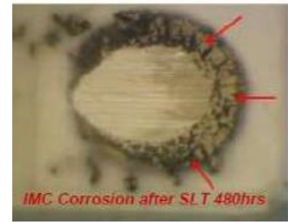
IMC Corrosion in Ag Wire on Al Bond Pad
