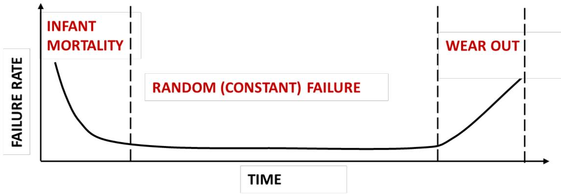
Figure 1: Example of a bathtub curve
