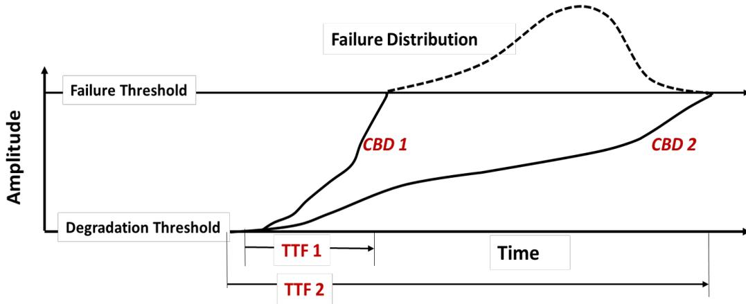
Figure 5: Degradation signatures: TTF relationship to failure distribution
