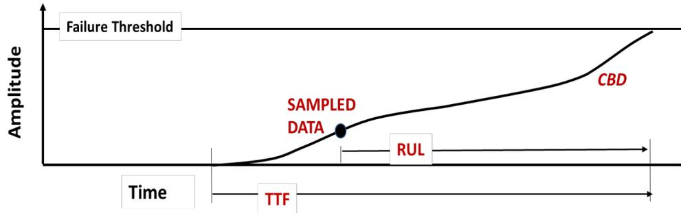
Figure 6: Degradation signature, TTF, sampled data, and RUL
