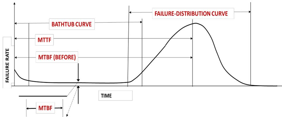
Figure 3: Combined bathtub and failure-distribution curve showing MTBF (between)
