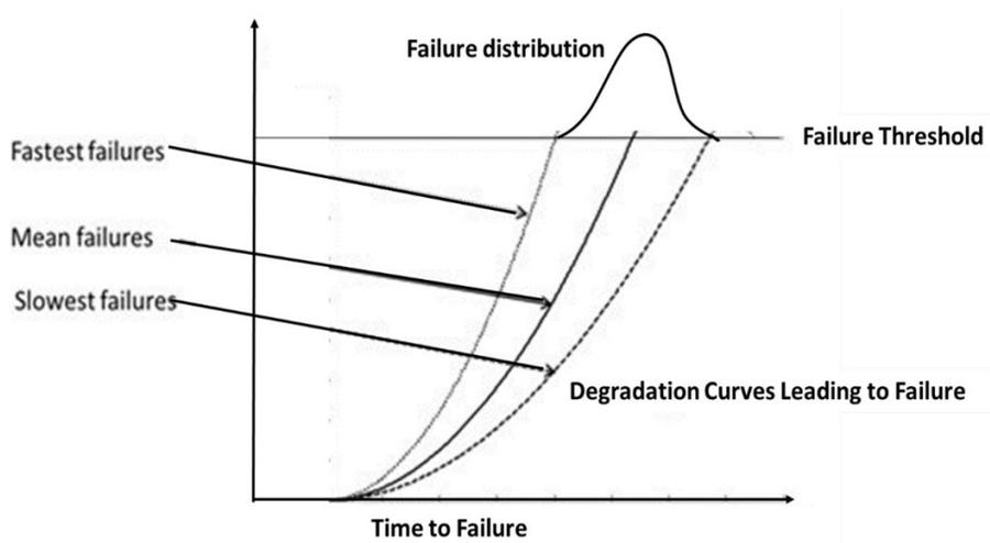
Figure 2: Example of a failure distribution curve due to degradation failures (wear out)
