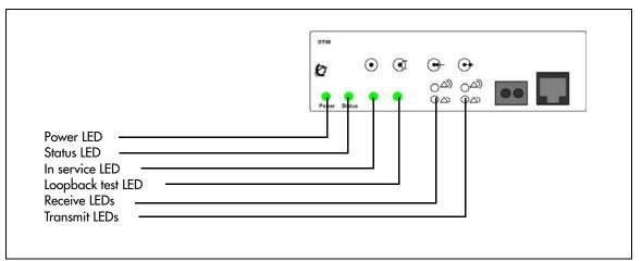
The table **DTM LED** functions on page 24 describes the functions of the DTM LEDs.
