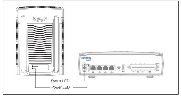
The table System status LEDs states and descriptions on page 18 describes the meaning of the system status LEDs after the system boots up and is in service.
