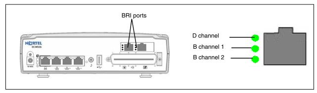
Figure 5 BRI port LEDs on the BCM50b, BCM50ba, and BCM50be main units (BCM50b shown)
