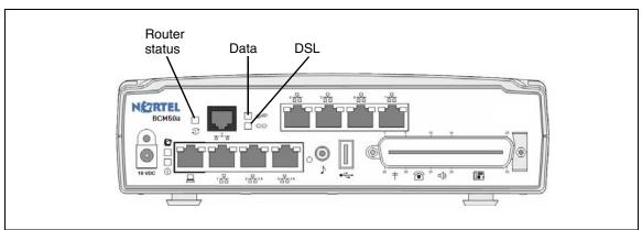
Figure 3 ADSL router LEDs on the BCM50a and BCM50ba main units (BCM50a shown)
