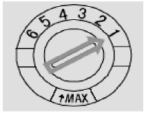
The rinse aid dispenser has six settings. ALWAYS START WITH THE DISPENSER SET ON "1". IF SPOTS & POOR DRYING ARE A PROBLEM, INCREASE THE AMOUNT OF RINSE AID DISPENSED BY REMOVING THE DISPENSER LID AND ROTATING THE DIAL TO "2". IF THE DISHES ARE STILL NOT DRYING PROPERLY OR ARE SPOTTED, ADJUST THE DIAL TO THE NEXT HIGHER NUMBER UNTIL YOUR DISHES ARE SPOT-FREE. \*\*\*NOTE: Please read the notes for detergent use on p. 13.
