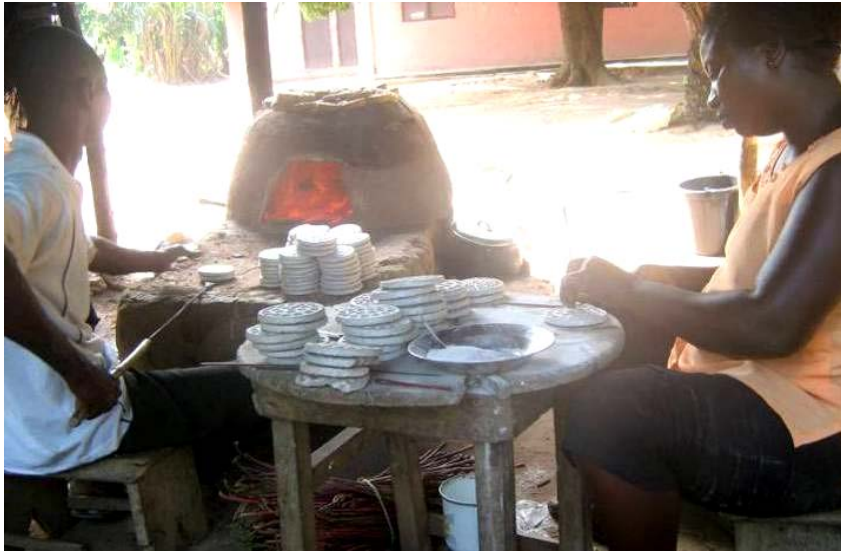
Plate 25: Powdered glass ready for the oven. (Picture by Researcher)
