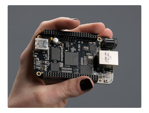
The BeagleBone Black includes a 2GB or 4GB on-board eMMC flash memory chip. It comes with the Debian distribution factory pre-installed. You can flash new operating systems including Angstrom, Ubuntu, Android, and others. The following pages will illustrate the steps to getting the latest of each type of supported distribution onto the on-board eMMC.
