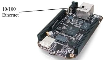
Figure 39. Ethernet Connector
