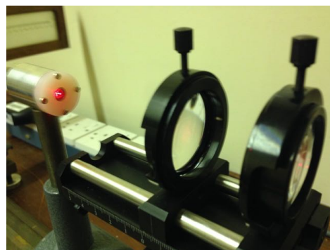
Figure 1.5: Laser spot focused onto photodiode
