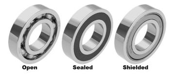
The capacity of a bearing will be the same regardless if is open, has seels, or shields. All three bearings will accept the same load and produce the same life. The three bearings will have different speed limits. Speed limits are determined by how hot the bearing will operate. The higher the
