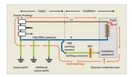
Protective Multiple Earthing (PME) has been almost universally adopted by DNOs in the UK as an effective and reliable method of providing their customers with an earth connection. This supply system arrangement is described in BS 7671 as TN-C-S.
