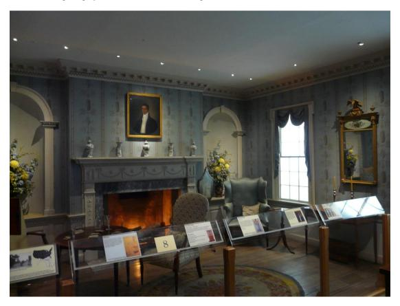
The American Museum in Britain, lit with eighteen 2 W adjustable LED downlights. These were positioned on the ceiling to light a given area or object well with a specific beam angle. For example, the long information panel at the front was lit by just three spots with elongation beams to give a long wide light spread.
