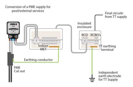
Once the TT arrangement has been formed with the appropriate earth electrode it is necessary to ensure that this system and any of the pool extraneous-conductive-parts are not connected to the PME earthing system by any 'casual' connection, as this would only serve to create problems.
