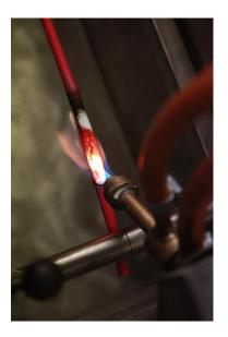
The Bunsen burner flame propagation test
