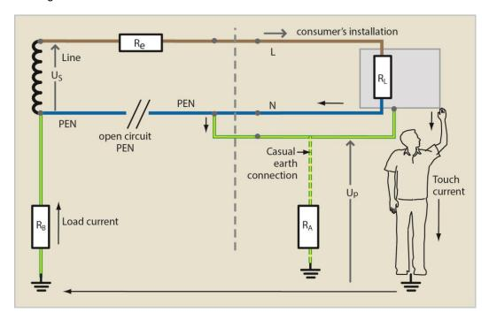
The touch voltage will be determined by the load connected within the installation and the value of the earth electrodes and any casual connections to earth that is provided by the bonded services.
