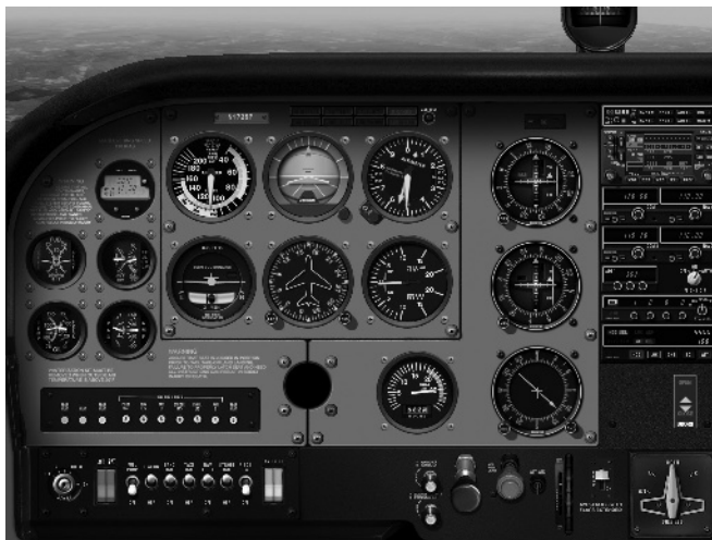
Figure 1-9: Default Cessna 172 Skyhawk instrument panel in X-Plane 9
