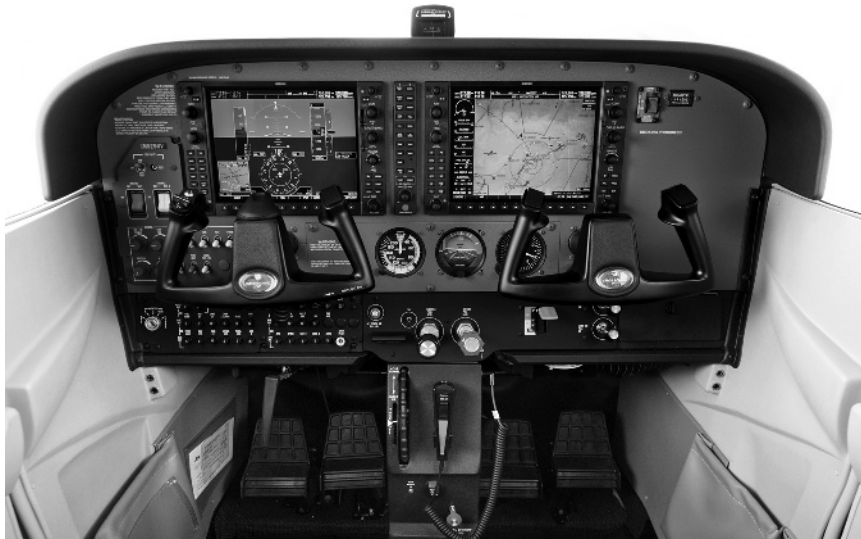
Figure 1-8: Garmin G1000 system in a late-model Cessna 172 Skyhawk
