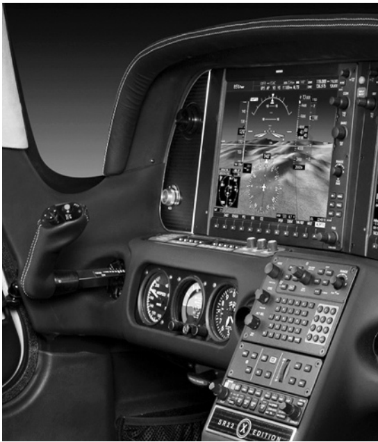
Figure 1-7: Side-stick control in a Cirrus SR22.
