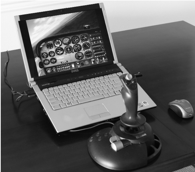
Figure 1-1: The minimum required setup for X-Plane or FSX: a laptop, mouse, and joystick
