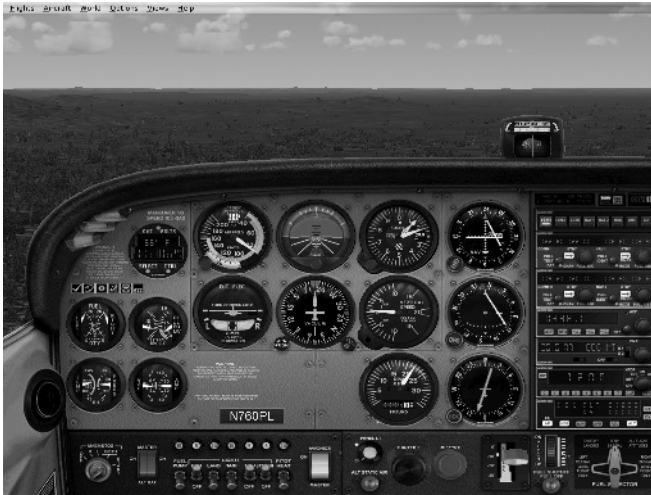
Figure 1-10: Default Cessna 172 Skyhawk instrument panel in FSX
