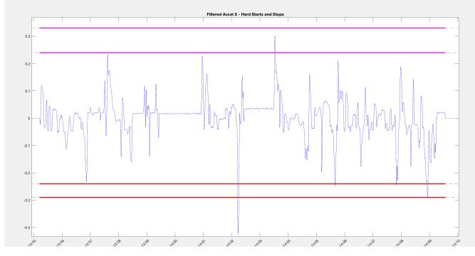
Figure 2. Kinematic events, consisting of hard starts and hard stops at different levels (purple and red lines, respectively) based on time series data, acceleration X.
