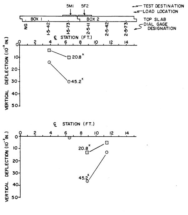
FIGURE 13. MEASURED VERTICAL DEFLECTIONS-CENTERLINE OF 5FT. SLAB 4.3 Discussion of Results
