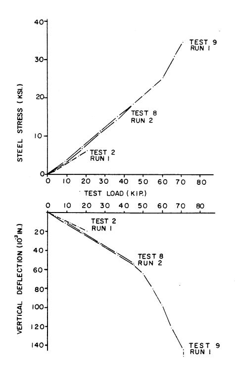
FIGURE 14. REPEATED LOAD-DEFLECTION DATA-STATION 1-7-73 TEST CONFIGURATION 7MI
