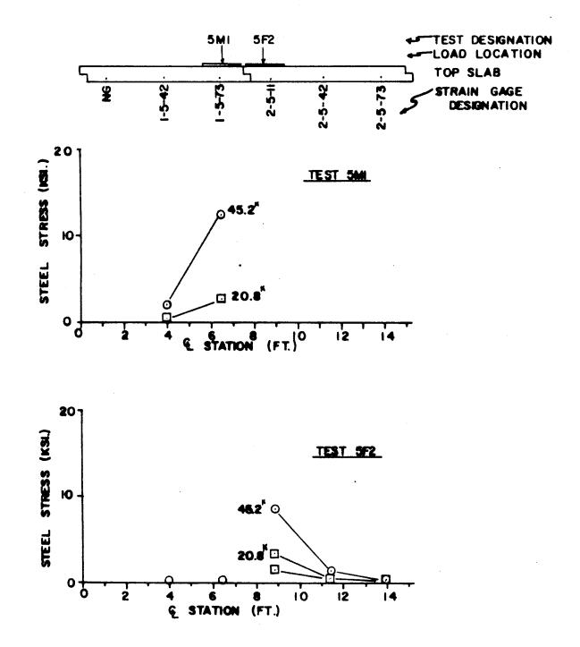
FIGURE II. MEASURED REINFORCING STEEL STRESSES CENTERLINE OF 5FT. SLAB
