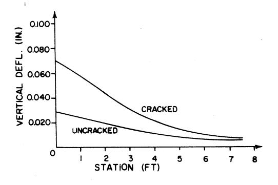
FIGURE 5. PREDICTED VERTICAL DEFLECTIONS CENTERLINE OF 7FT SLAB
