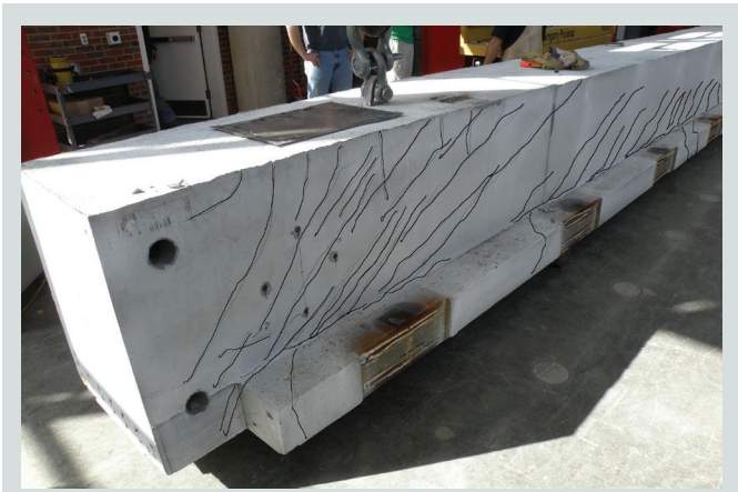
Figure 6. Inner face cracking observed after failure for a compact L-shaped beam with open web reinforcement (LG4). Note: Cracks are digitally enhanced.
