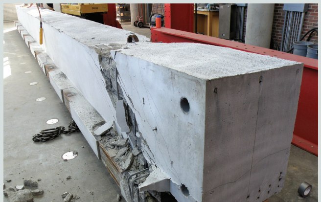
LG4 (C-shaped inner-face reinforcement)
