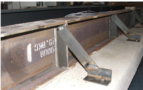
Fig. 2. Bracing used to eliminate lateral-torsional buckling.
