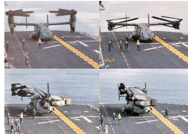
Blade Fold/Wing Stow Sequence
