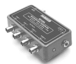
Models MC102, 104, 202 and 204 are passive couplers, and therefore need no external power to operate. However, because of the passive design each coupler will exhibit some signal loss from input to output ports. A 2-port device has slightly more than 3 DB signal loss, and a 4-port slightly more than 6 DB loss. On a receiver with a calibrated S-meter this will result in a reduction of meter reading of 1/2 S-unit for a 2 port coupler and about one S-unit for a 4-port coupler.
