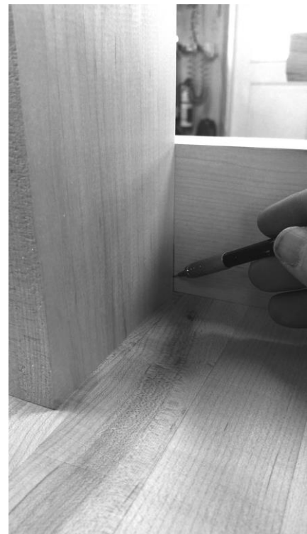
Scribe the rail's tenon shoulder from the inside of the leg.
