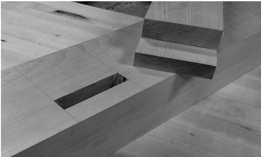
The completed rail mortise and tenon.
