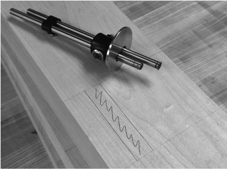
Layout the eight mortises in all four legs
