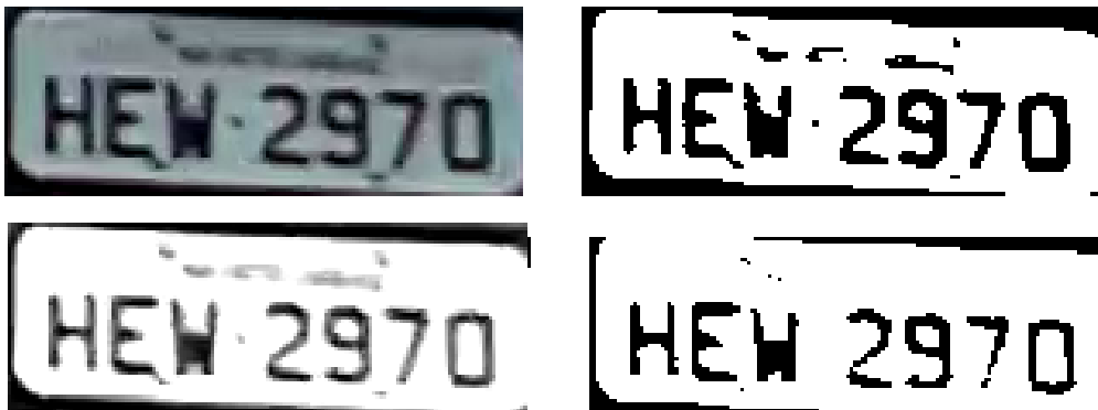
Fig 5 Comparison between images. Original image (top left), binarized by Otsu method (top right), binarized by IGT method (bottom left) and binarized by the proposed iterative approach (bottom right).
