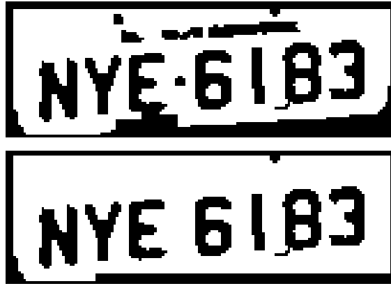
Fig 2 At the top there is an example of an image binarized without the SL*L preprocessing and at the bottom an image binarized using the SL*L processing method.
