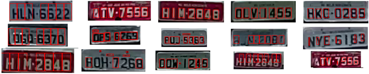
Fig 15 Examples of the segmentations by each baseline. First column shows license plates segmented by the Prior-Knowledge approach. Second column shows license plates segmented by CCL approach. Third column by SLL approach. Fourth column by IGT approach. Fifth column by the proposed iterative approach.
