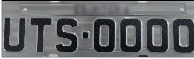
Fig 1 Example of the Brazilian license plate standard. It is composed by two rows: in the first one, the acronym of state followed by its origin city (blurred in the image); in the second row, under the first one, there are three letters one blank space or hyphen and four digits to identify the vehicle.
