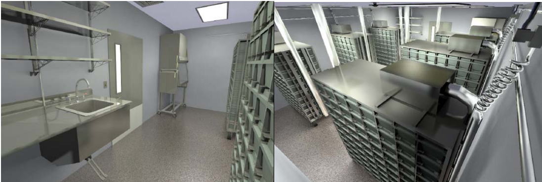
Figure 19: Animal Holding Room 703B Rendering - Stainless Steel Casework, Animal Transfer Station, Cages Animal Watering system, epoxy flooring, etc.
