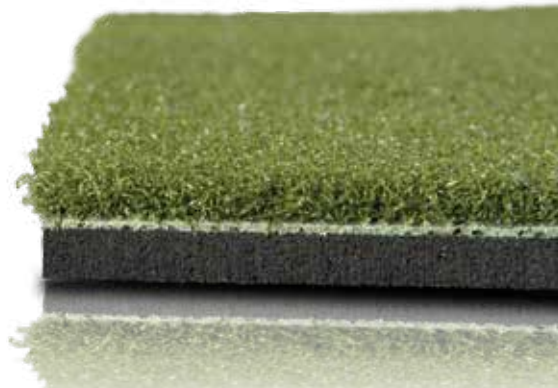
5mm or 12mm rubber backing. Turf wear layer and rubber backing work together to create an acoustically ideal product: absorptive on top, vibration isolating on bottom.
