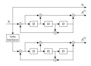
Fig. 2. LTE rate 1/3 turbo encoder [17].
