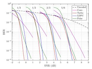
Fig. 11. BER comparison for different code rates, K=1024 (For LDPC, K=1020 for  $R=1/2, 1/3, \mbox{ and } 5/6.)$
