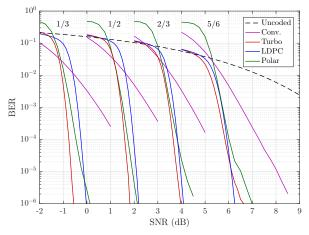
Fig. 12. BER comparison for different code rates, K = 2048 (For LDPC, K = 2052 for R = 1/2, and 1/3, and K = 2040 for R = 5/6.)
