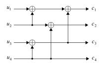
Fig. 4. Polar encoder of length 4.
