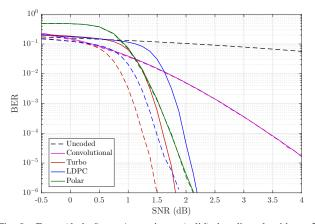
Fig. 8. Exact (dashed) vs. Approximate (solid) decoding algorithms, K = 2048 (2052 for LDPC), R = 1/2, 8 iterations turbo, 16 iterations LDPC, list size 8 polar.
