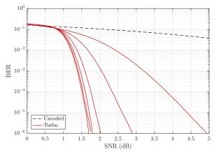
Fig. 5. Turbo code convergence, K = 2048, R = 1/2, Iterations = 32, 16, 8, 4, 2, 1 from left to right.
