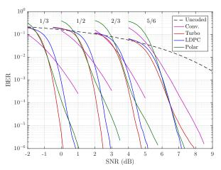
Fig. 10. BER comparison for different code rates, K = 512 (For LDPC, K = 516 for R = 1/2, and 1/3, and K = 520 for R = 5/6.)
