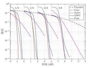
Fig. 13. BER comparison for different code rates, K = 4096 (For LDPC, K = 4092 for R = 1/2, and 1/3, and K = 4100 for R = 5/6.)
