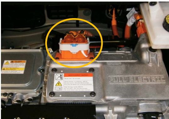
Vehicle not fitted with rapid charging
