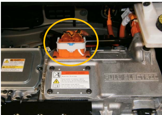
Vehicle not fitted with rapid charging
