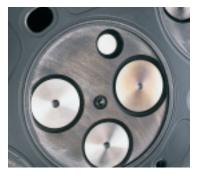
The engine breathes better with three valves per cylinder. A fourth valve is utilized for the optional MBE 900 compression brake.
