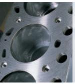
Cylinder bores are inductionhardened around the upper piston ring area, and when combined with special coatings on the rings themselves, overall durability is improved.
