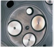
The engine breathes better with three valves per cylinder. A fourth valve is utilized for the optional MBE compression brake.
