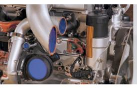
The oil and fuel filters are positioned upright in front of the engine for ease of service and maintenance.
