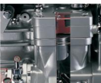
The gear-driven air compressor uses 50 percent less power, leaving more power for driving and helping to reduce fuel bills.
