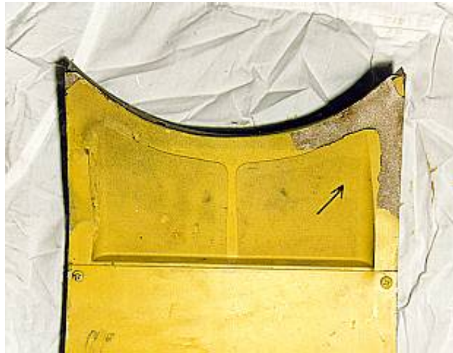
Figure 1. Corrosion Damage Resulting From Moisture Entrapment Under a Failed Non-Load-Bearing Adhesive Bond Applied After Minimal Surface Preparation
