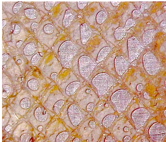
Figure 22. Microvoiding in Moisture-Contaminated Adhesive Cured Under Vacuum (Square shapes are carrier cloth with 0.020-inch pitch.)
