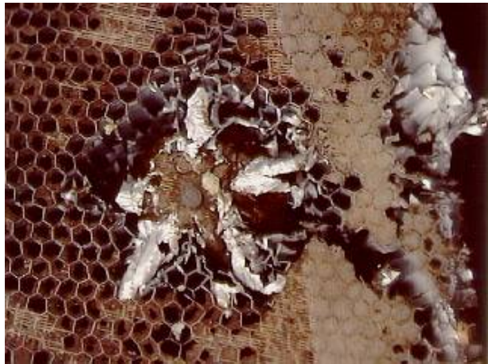
Figure 20. Corrosion Damage due to Previous Injection Repair in Honeycomb Sandwich Panel
