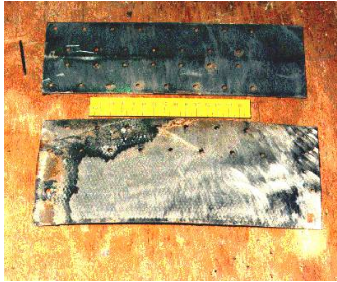
Figure 14. Photograph of Patch That Suffered Adhesion Failure in Service
