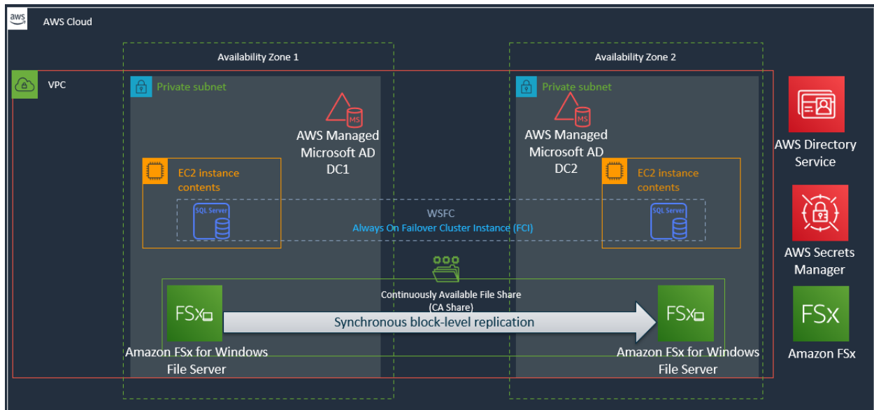
Figure 2: AWS Launch Wizard deploys MS SQL FCI using Amazon FSx for Windows File Server
