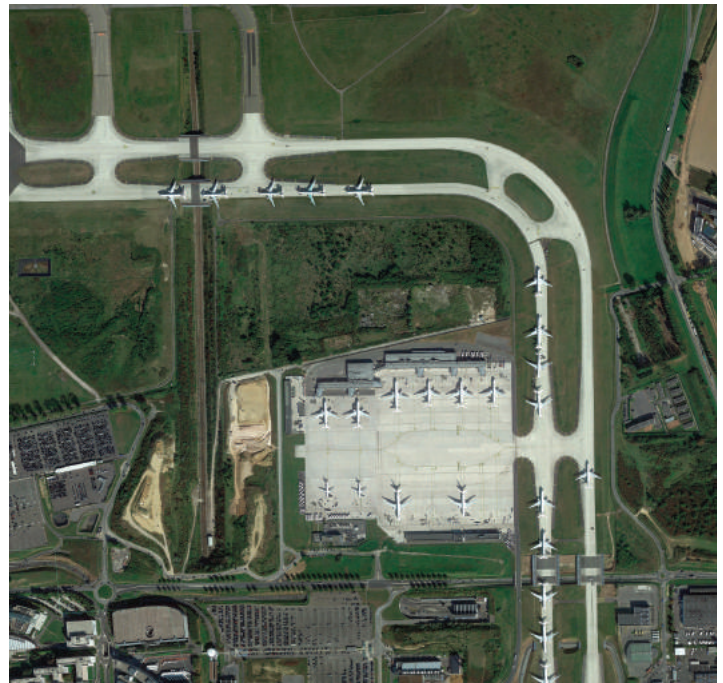
Figure 3 Temporary parking of overflow aircraft on Taxiways CHARLIE and BRAVO at Paris-CDG (2014)
