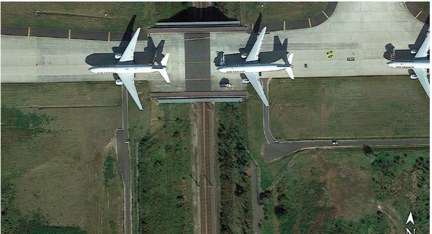
Figure 4 Bridge friendly parking of overflow widebody aircraft (CDG, 2014)
