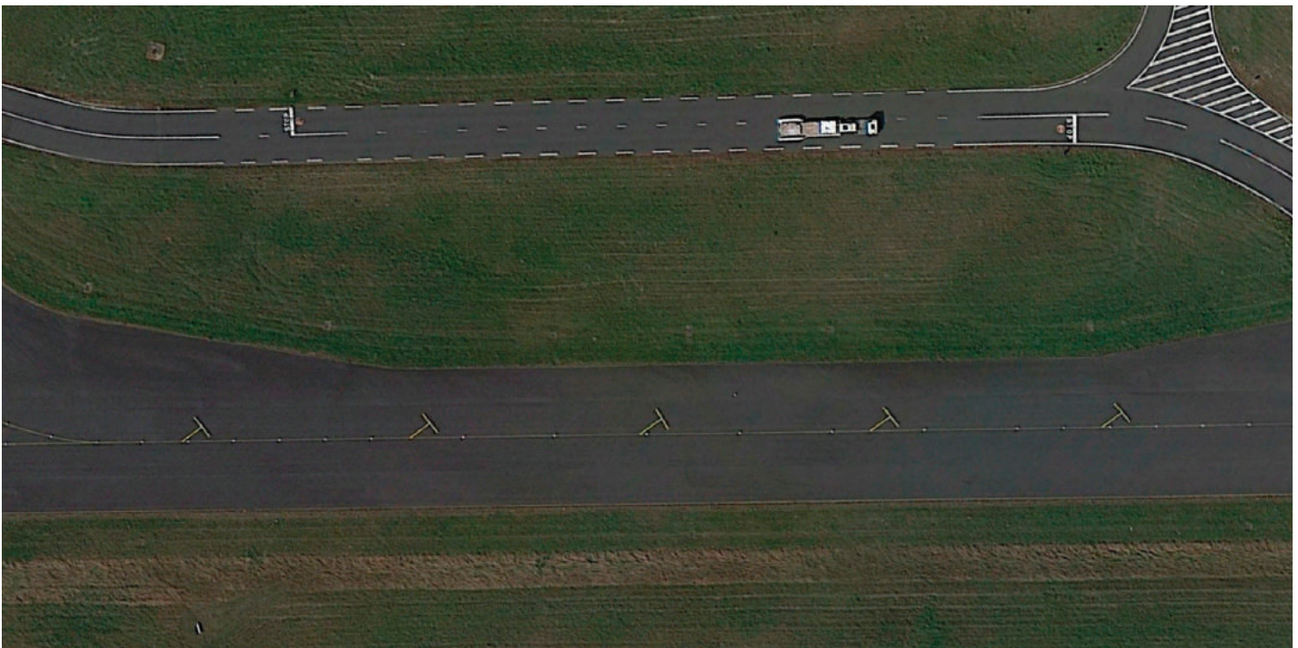
Figure 1 “T markings” for overflow A320 family aircraft parking on Taxiway CHARLIE at Paris-CDG (2014)
