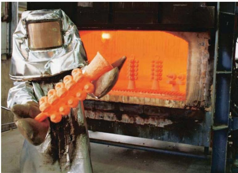
It takes eight minutes to heat 27kg of stainless steel to the 1500°C required for casting.
