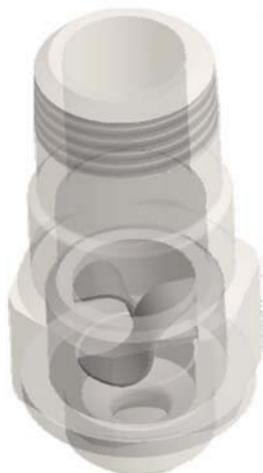
A cutaway view of the MaxiPass nozzle showing the S-shaped vanes that enable the nozzle to successfully handle large particles without clogging.
